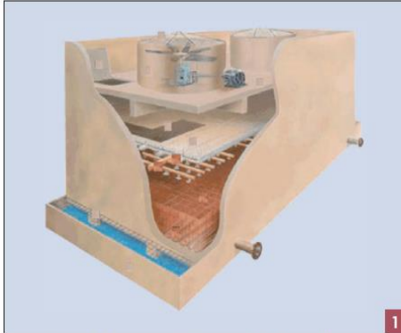
Typical cooling tower arrangement with two cells.
